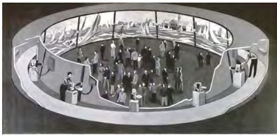
Eleven projectors are electrically synchronized to show one continuous picture on the "Circarama" theater screen
